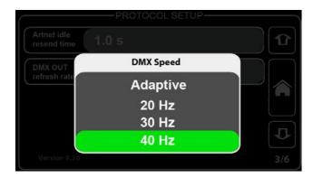
Select one of four options for "DMX out refresh rate" (Adaptive, 20Hz, 30Hz, 40Hz).
