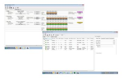
ProPlex IQ Ethernet to DMX nodes can also be remotely configured via their onboard webserver. Using a PC or Mac internet browser, connect to individual IQ nodes by typing their IP address into the internet address bar.
