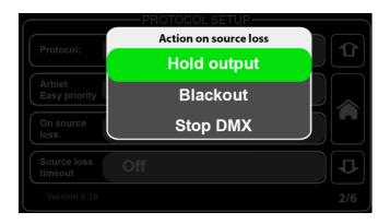
When the "**Hold values**" setting is chosen, after the source DMX is lost, the IQ Two 1616 2x holds the last DMX values it has received and continues to output these values until incoming DMX has been restored.
