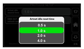
This setting determines the time Art-Net will refresh the signal after idling. Select from 0.5s, 1s, 2s or 4s, depending on the requirement. This only applies to ProPlex IQ Two 2x DMX connectors set to input mode. Some consoles may not resend a DMX packet if there is no change in the value. Art-Net idle resend time ensures Art-Net regenerates the unchanged value as some devices — e.g. media servers and moving lights — need recurring DMX over Art-Net even if no change in values exist.
