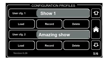
In the main Configuration Profiles screen, either load or delete the configuration saved.
