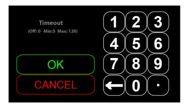
This setting determines how long the IQ Two 2x will wait before using the Source Loss setting. This time is set in seconds (5-120). Once the source loss timeout time has been reached, the IQ Two will revert to the Source Loss timeout setting.
