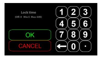
Here screen lock time may be set. This setting will change the time after which the ProPlex IQ Two will lock the screen.
