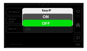
This setting ensures that software will search for all masks, not just the one specified. If Easy IP setting is turned ON, the Subnet Mask cannot be changed. Easy IP is very useful for most networking situations where subnet filtering is not required. The IQ Two 1616 2x will automatically find and output Art-Net and sACN information regardless of IP or Subnet Mask settings.
