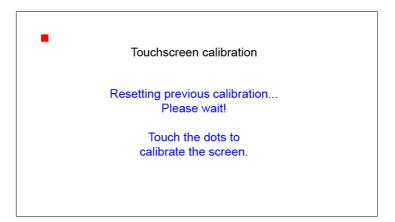
Press the red dots to calibrate the touchscreen. There will be four dots in total, each dot in all four corners.
