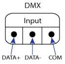
2.1 To pass DMX to another device, connect the DMX cable to the DMX Thru port located in the right top corner of the unit. The connector should be wired as depicted in the image below.
