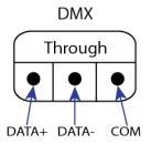
3. Connect the optically isolated DMX signal outputs to DMX links. The connector should be wired as depicted in the image below.
