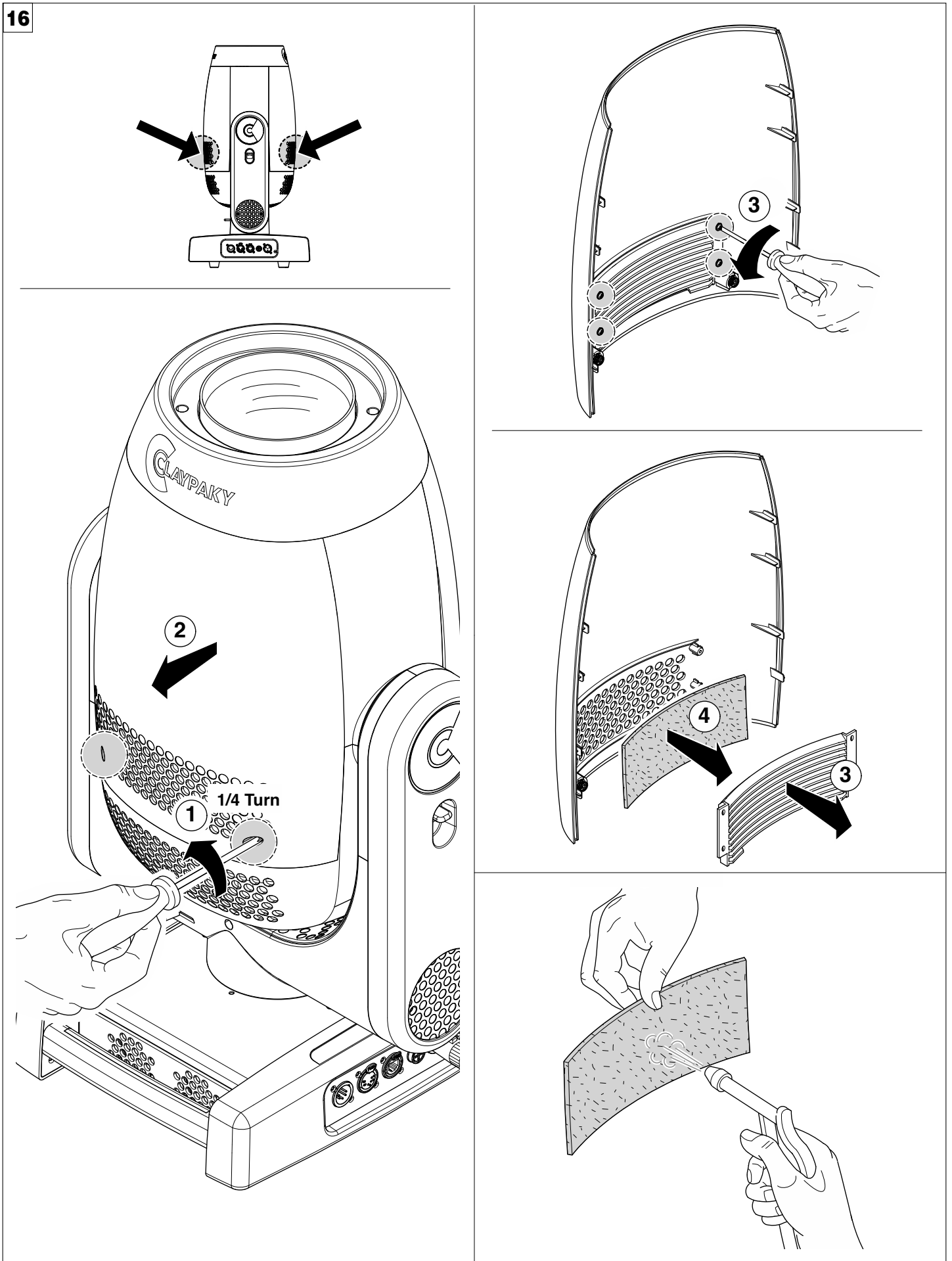
Cleaning of the filters - Fig. 16.
