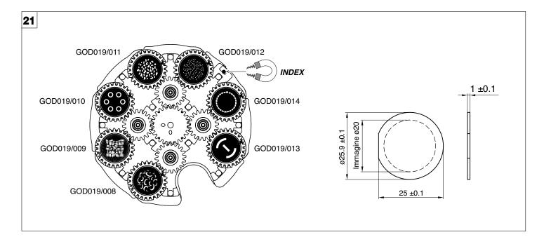
Replacing rotating gobos (max 20 mm image – thickness 1 mm) - Fig. 21
